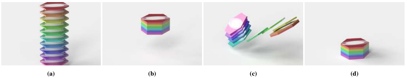
Figure 7: Stacked permanent magnets. (a) Initial state. (b) An intermediate simulation result: The magnets are strong enough to be stacked in the air. (c) In EDM, the excessively strong forces and torques cannot be prevented. (d) MBM produces stable simulation results.
